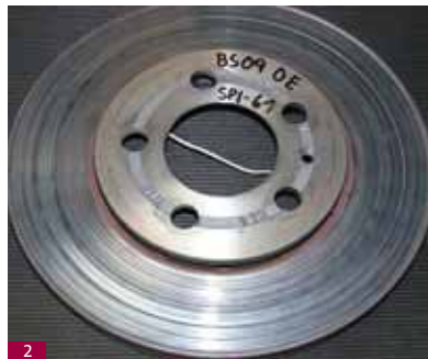
1 An NK brake disc in the second series of tests after 438 braking cycles. It is already completely cracked.
