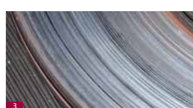
3 A Volkswagen brake disc in the last series of tests after 440 braking cycles. Only light cracks of up to 25 mm are evident.
